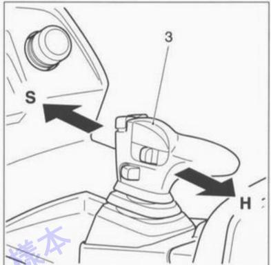
The safety switch installed is an active accident prevention device which protects the truck against accidental acceleration with a raised load outside the free lift range.
